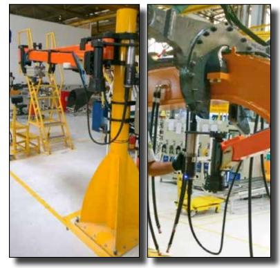
Final Assembly Tightening Car Swing Bearing
