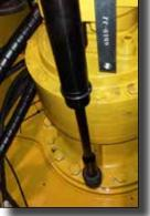
Wheels to Hub 2 step tightening 12 bolts Torque 1 = 200 nm Torque 2 = 600 nm
