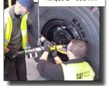
Counterweight Target Torque = 2800 nm System on portable base (moved by tug). Reaction arm absorbs torque reaction.
